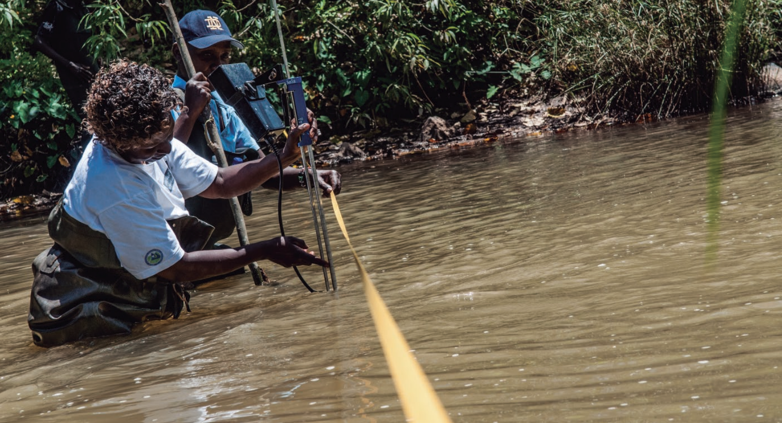
Measuring river discharge in Kenya. Photo/Georgina Smith
